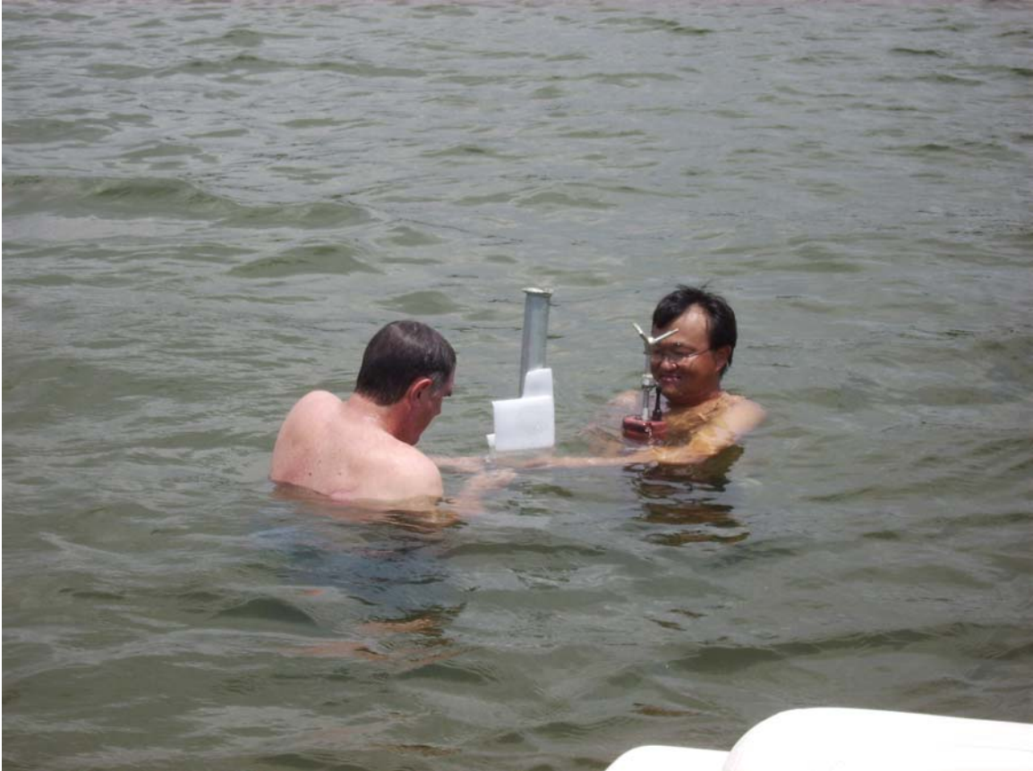
Figure 3. Installation of the Triton wave gage at Site 1.
